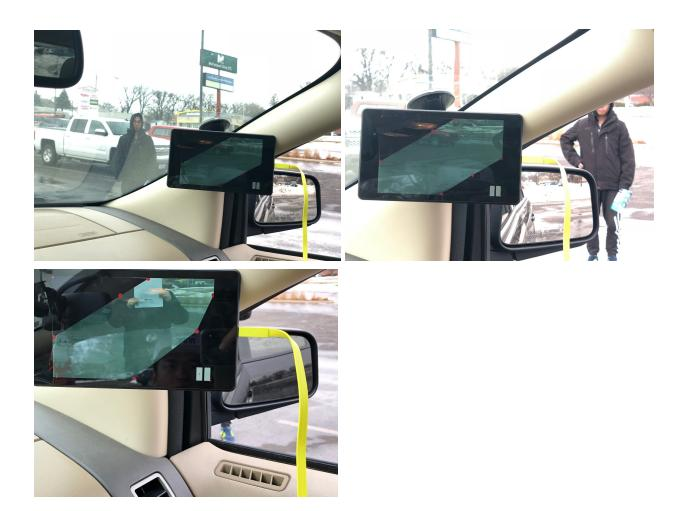
Figures: The photos we took during testing. We tested the largest angle of view as shown in first two pictures. The tester held a paper with letter on it and we test out the longest distance of visibility as shown in the third picture.
